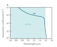
Through the integration of GeSi (Germanium-on-Silicon) as the light absorption material with CMOS technology on silicon wafer, Artilux has successfully extended the available sensing spectrum up to 1550nm. This disruptive technology platform was developed in collaboration with TSMC, thereby ensuring the sensor quality and reliability in the production stage.
